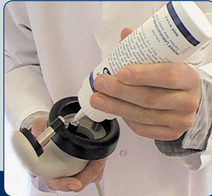
Apply a drop of electrode gel on each of the three BERAphone® electrodes.
